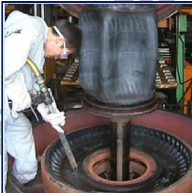
An opened tire mold being cleaned. The deflated rubber bladder is on the central post.
